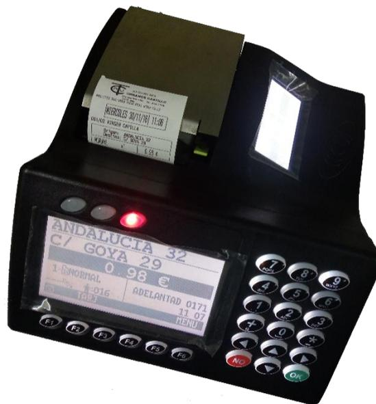
This machine, despite being small in size, incorporates a large screen and an industrial backlit keyboard to interact with the driver. It acts like central computer of the installation and manages all the elements embarked.
